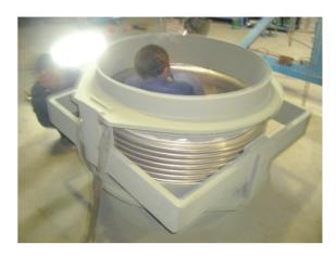
Typical gimbal systems consist of two gimbal expansion joints or two gimbal and one hinged expansion joint
